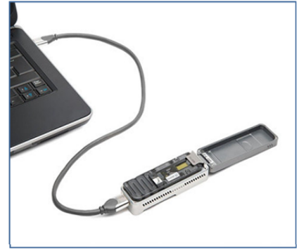
Oxford Nanopore's MinION™ USB-attached miniature sensing device
